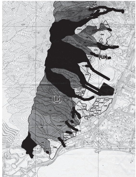
Figure 12. Hazard map delineating (a) areas potentially affected by debris flows; (b) zoning of catchment based on risk of debris flows on downstream development, i.e. with consideration of susceptibility and consequence of debris flows
