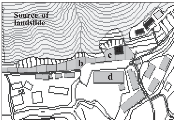
Figure 13. Risk zoning map from QRA showing annual risk in terms of potential loss of life x 10,000 - (a) 2 - 5; (b) 0.2 - 0.5; (c) 0.02 - 0.05; (d) < 0.02 (based on OAP, 2003)
