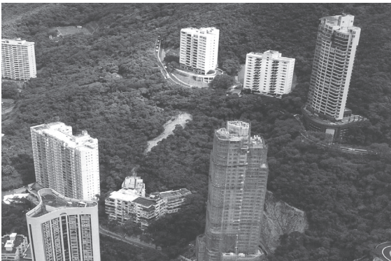
Figure 3. A 50 m 3 landslide in 1998 resulted in damage to property
